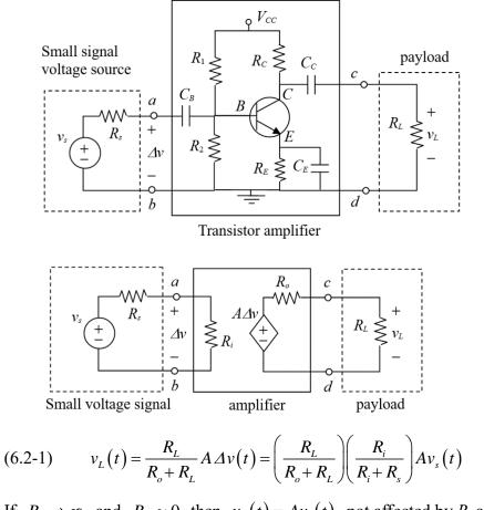
If  $R_i \to \infty$  and  $R_o \approx 0$ , then  $v_L(t) = Av_s(t)$ , not affected by  $R_s$  and  $R_L$ .
