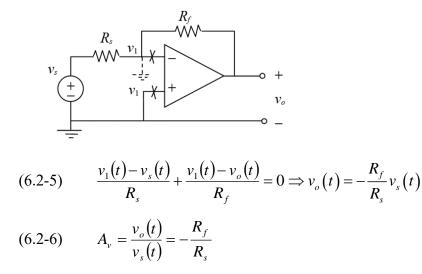
The voltage gain is negative and called the inverting amplifier. Example: If  $R_L = 1 \text{ k}\Omega$ , what is  $i_L(t)$ ?
