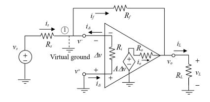
$$(6.2-2) \qquad R_i \to \infty, \quad R_o \approx 0, \quad , \quad A \to \infty, \quad ,$$
